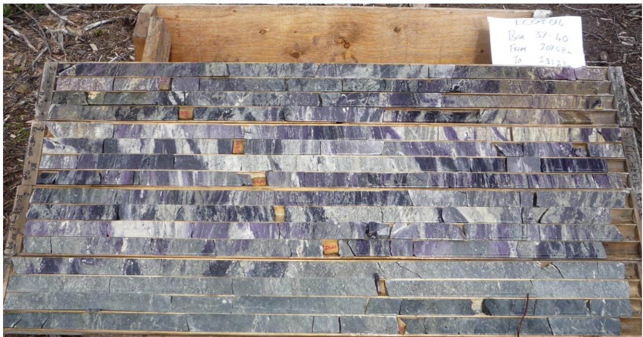
Figure 1: Section of high-grade fluorspar zone in drill hole EC08-016
